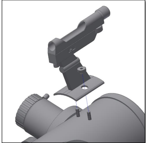
Figure 11. Place finderscope and thread the thumbnuts
