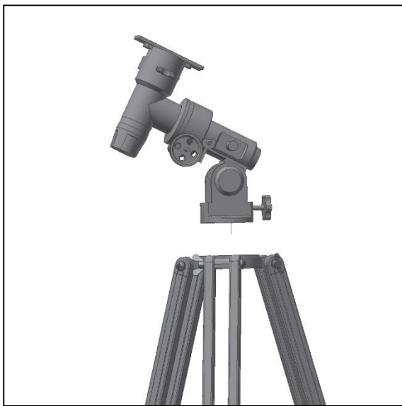
Figure 4. Place the equatorial head.
